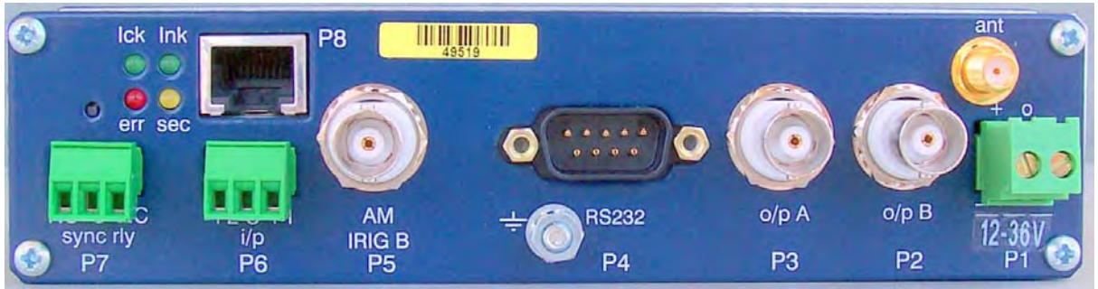
Figure 2. Rear Panel of the XL-750, Rev D, with BNC and NTS Output Options
