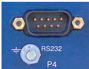
Figure 5. P4 - RS232 Port and Ground Stud
